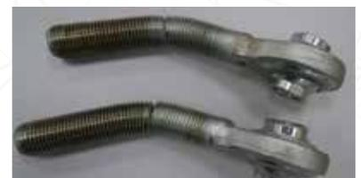
» Bending test on the top link spindles up to a bending angle of approx. 30°
